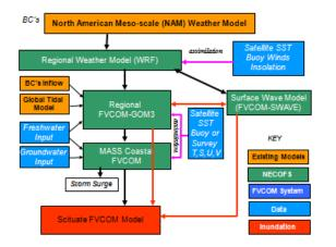
**Figure 1** Schematic of NECOFS, showing the three core models (WRF, FVCOM 3.1, SWAVE). Note that the Scituate FVCOM inundation forecast model system can be driven by either FVCOM-GOM3 or MASS Coastal FVCOM.
